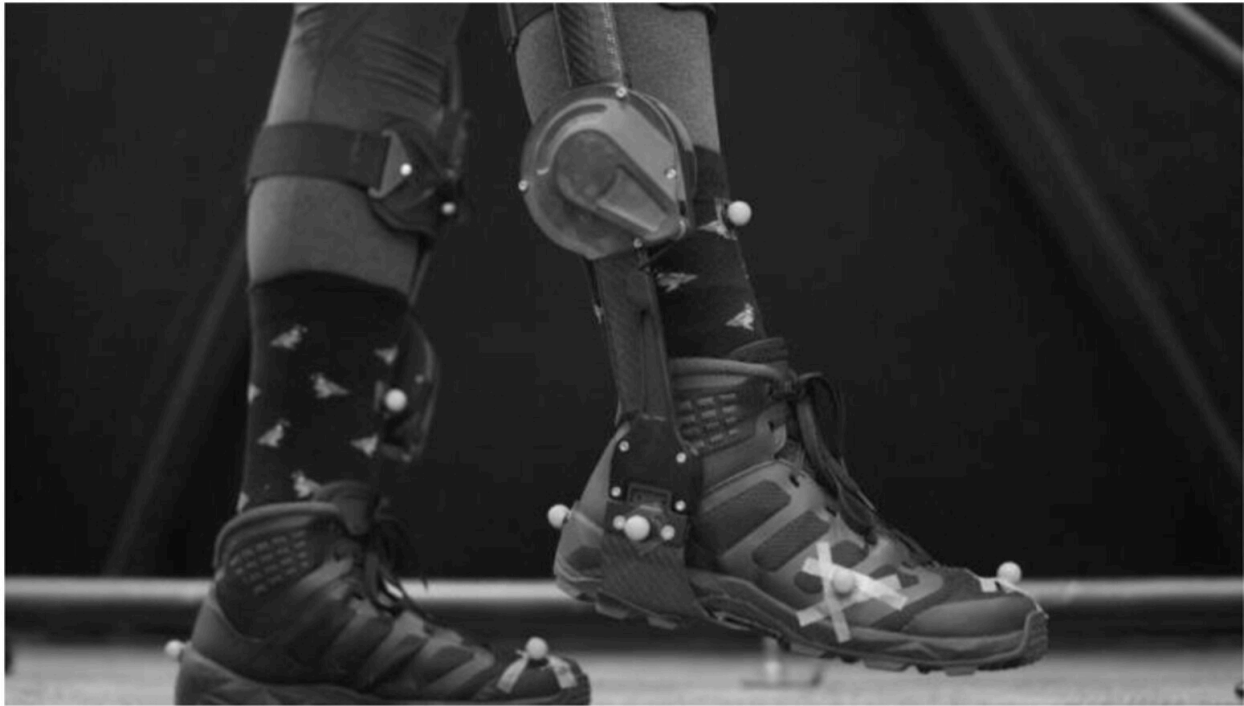
Figure 5. Demonstration of the Dephy ExoBoot (DpEp45 exoskeleton which shows a carbon fiber footplate combined into an ankle-high boot. The footplate is attached to a shank-mounted assembly consisting of a unidirectional actuator (51).
