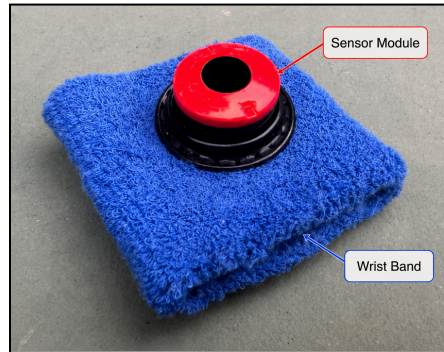
Figure 3: IMU-Based Sensor Integrated with the Wrist Band
