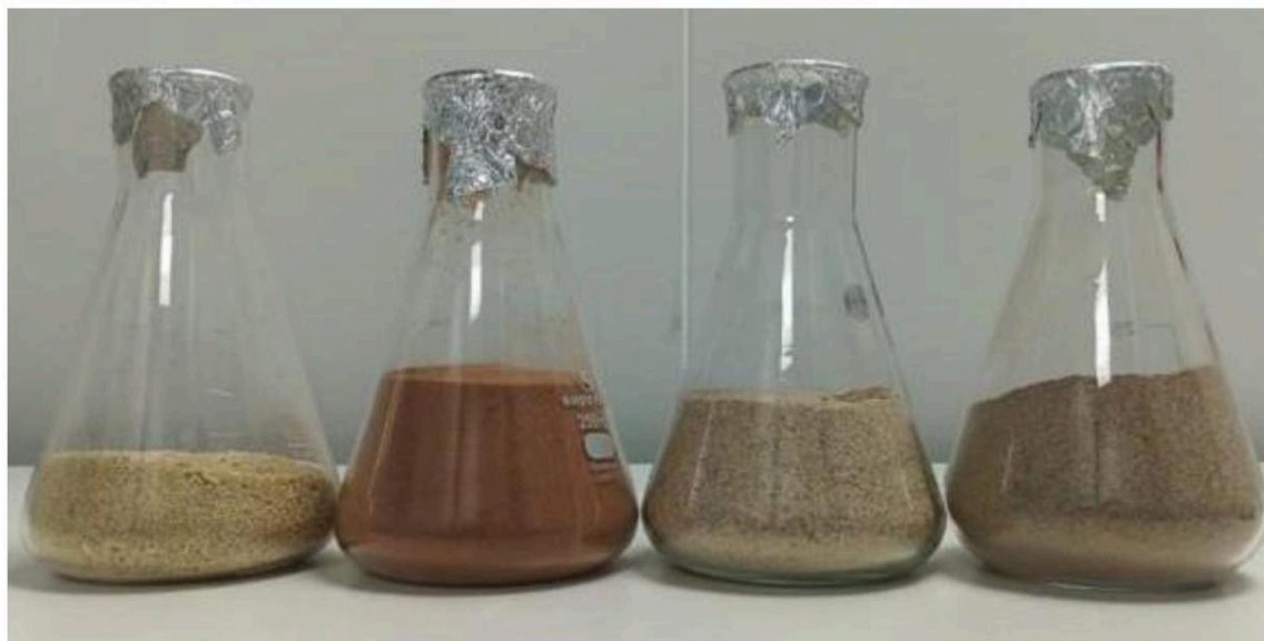
Figure 1. Agro-based lignocellulosic substrates (From left to right: Napier grass, coconut husk, banana stem, and ragi stem) after drying and pulverization, prepared for use in SSF experiments.
