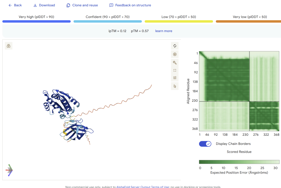
Figure 11. AlphaFold prediction of Caplacizumab, G101Y bound to vWF. iPTM score of 0.12 indicates low confidence in vWF-Caplacizuman interaction. pLDDT scores are greater than 90 in the folded A1 domain of vWF and <70 for the CDRs of Caplacizumab. Expected position error is high for Caplacizumab relative to vWF.
