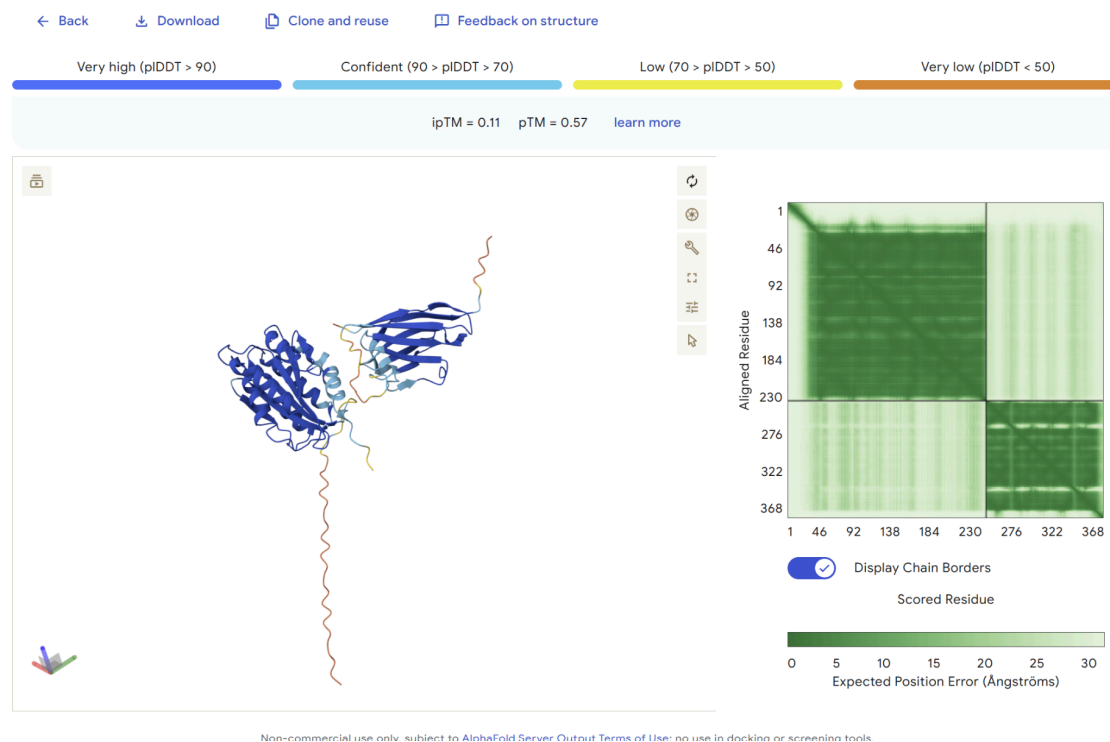
Figure 12. AlphaFold prediction of Caplacizumab, G101W bound to vWF. iPTM score of 0.11 indicates low confidence in vWF-Caplacizumab interaction. pLDDT scores are greater than 90 in the folded A1 domain of vWF and <70 for the CDRs of Caplacizumab. Expected position error is high for Caplacizumab relative to vWF.
