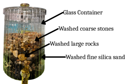
Figure 7: Materials used in the construction of the biosand filtration system.
