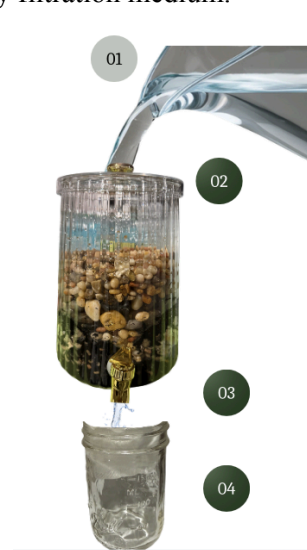
Figure 8: Step-by-step illustration of the water flow through the biosand filtration system during testing.
