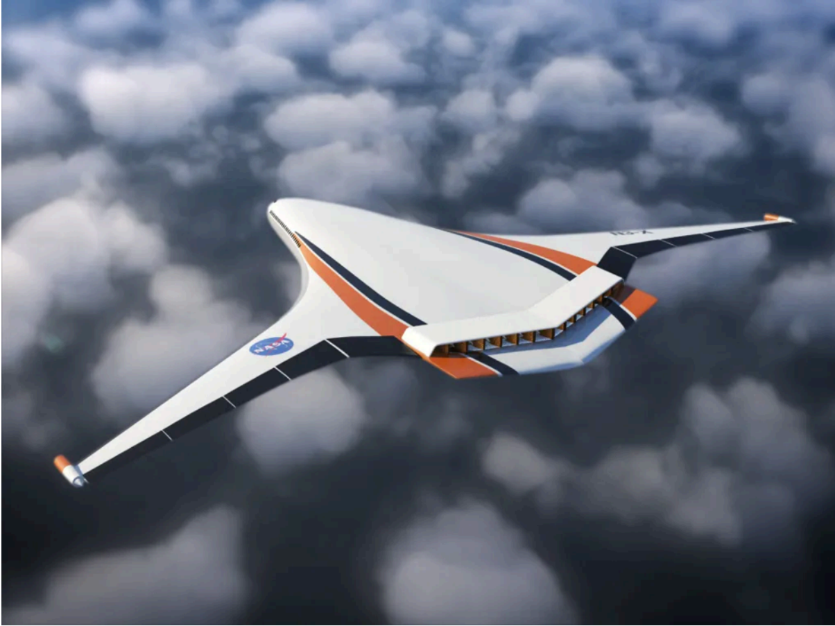
Figure 4 shows an airframe designed to shield the ground from noise while optimizing fuel efficiency.
