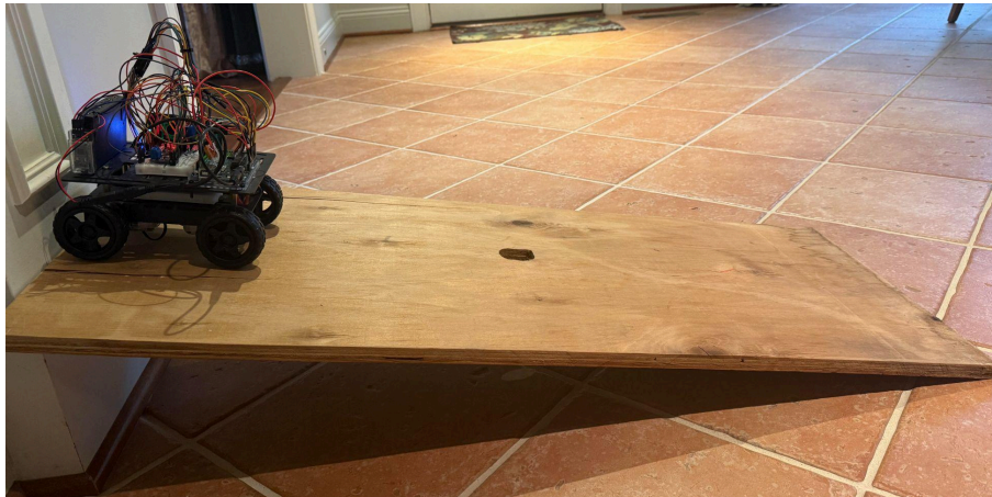
Figure 3. Experimental test setup showing the four-wheel-drive robotic platform positioned at the top of the adjustable wooden ramp prior to each trial. The adjustable ramp enabled controlled evaluation of regenerative braking under multiple incline conditions while maintaining a consistent test surface.
