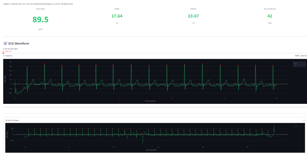
Figure 2. Real-time ECG Biosensor Dashboard showing live BPM, SDNN, RMSSD, peak count, and ECG waveform with R-peak markers.
