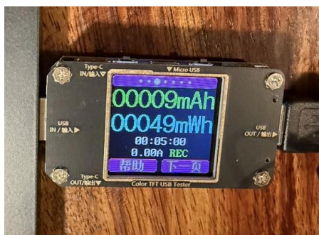
Figure 6: Energy measuring device showing energy consumption after 5 minutes
