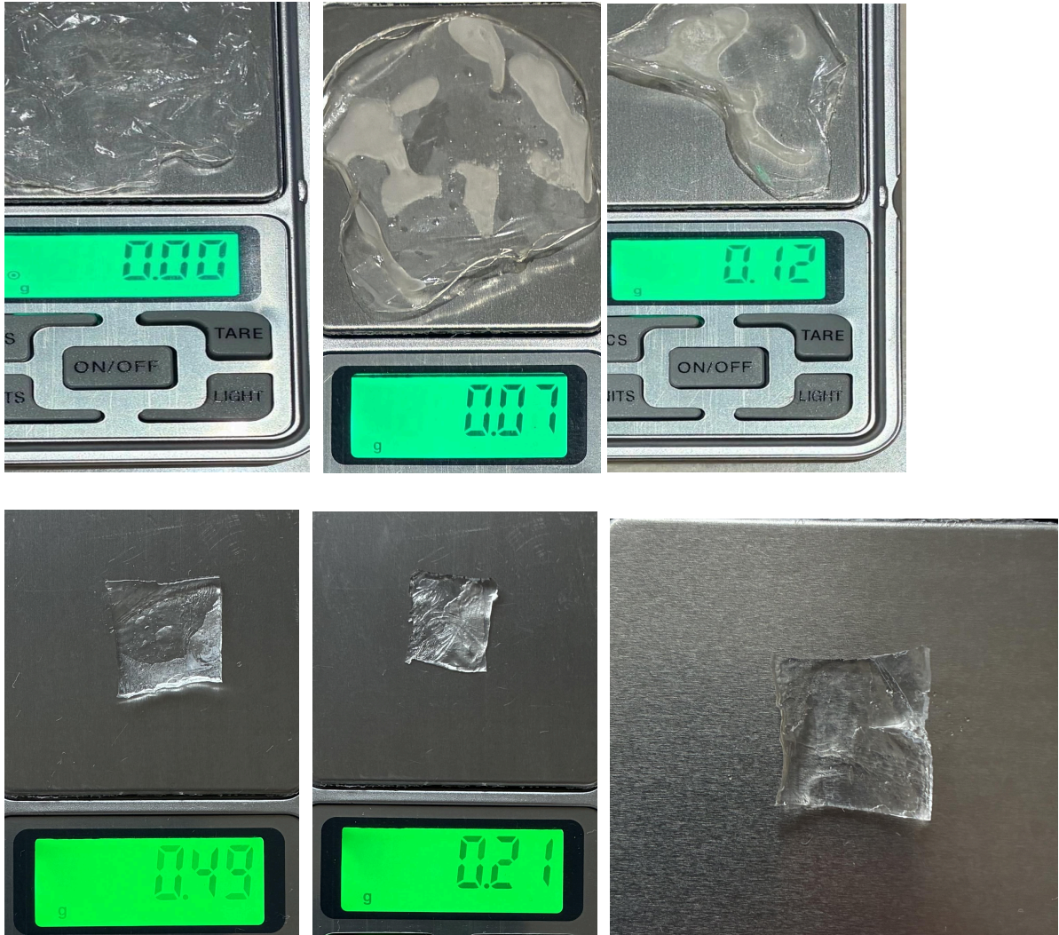
Figure 2. Water-uptake testing: hydrogel squares weighed on a digital kitchen scale (0.1 g resolution) before and after sequential water dosing (Table 2).
